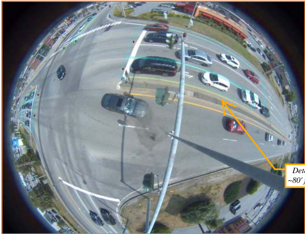
Example Zone Design for Gridsmart Detection System Maine Mall Rd at Gorham Rd, South Portland ME
