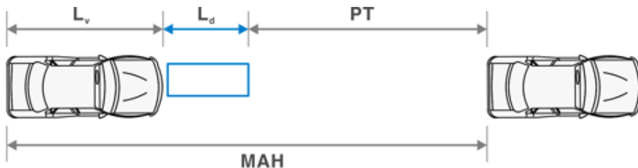
Figure 5-4 FHWA Signal Timing Manual L v : Length of Vehicle L d : Length of Detector PT : Passage Time = Extension MAH : Maximum Allowable Headway
